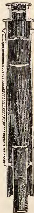
Draw-tube fitted with Erector.
